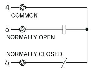
Auxiliary contacts are rated 15 amperes at 125, 250 or 480 volts AC; 0.5 ampere at 125 volts DC; 0.25 ampere at 250 volts DC. DO NOT EXCEED THE RATED VOLTAGE AND CURRENT OF THE CONTACTS. Contact operation is shown in the following chart:
